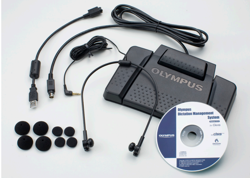
The kit includes the 4 pedal foot switch, headset, and Olympus Dictation Management System (ODMS) software.
